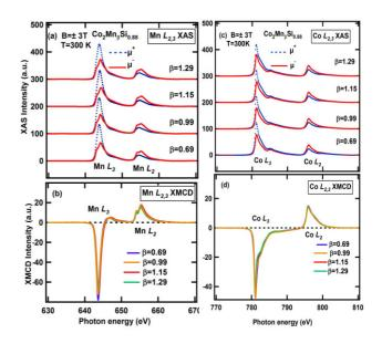
Figure 1(d) displays the Co  $L_{3,2}$ -edge XMCD spectra. For all the samples, a shoulder-like structure was observed in the higher energy region of the Co  $L_3$ -edge XAS as shown in Fig. 1(c). This feature is common to bulk samples [3]. The XMCD signals very slightly decreases as the Mn composition increases. We could not find CoO-like multiplet structure [4] for all the samples.
