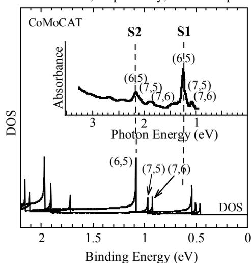
**Figure 1** Optical absorption spectrum of the CoMoCAT sample and the calculated densities of states (DOS) of (6, 5), (7, 5) and (7, 6) tubes.
