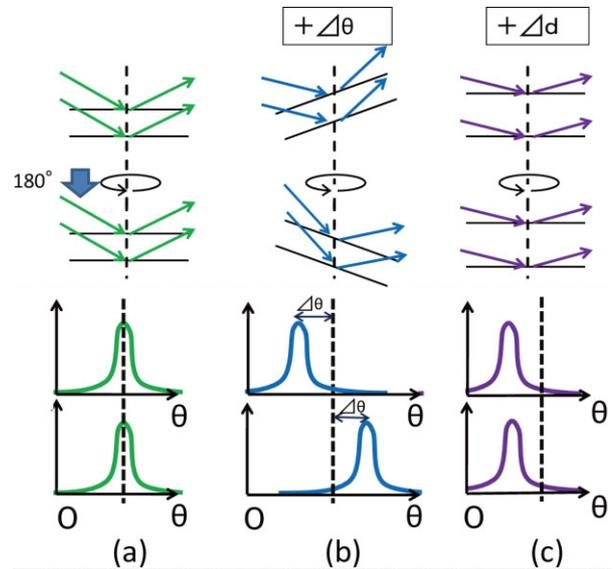
Fig. 1. Experimental principle of separation of  $\Delta\theta$  and  $\Delta d$ .
