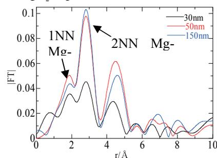
Fig. 1 Fourier transforms of  $\chi(k)$  for horizontal direction of MgB<sub>2</sub> films
