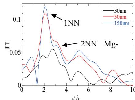
Fig. 2 Fourier transforms of  $\chi(k)$  for vertical direction of MgB<sub>2</sub> films
