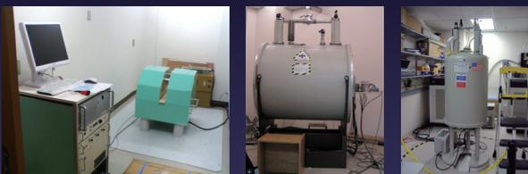
1.5T magnet (permanent)      2.34T magnet (super-conducting)      7T magnet (super-conducting)
